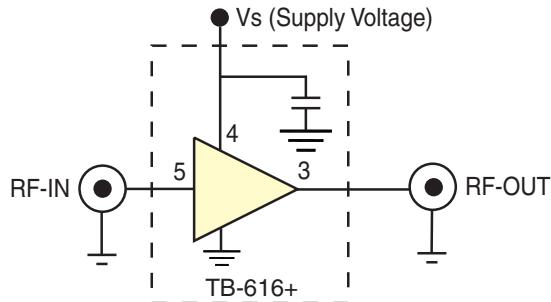
**Fig 1.** Block Diagram of Test Circuit used for characterization. (DUT soldered on Mini-Circuits Characterization Test Fixture TB-616+) Gain, Return loss, Output power at 1dB compression (P<sub>1</sub> dB), Output IP3 (OIP3) and Noise Figure measured using Agilent's N5242A PNA-X microwave network analyzer.
