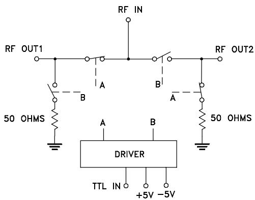
2. All RF connections must be blocked or held at 0V DC. Low frequency is determined by value of Coupling capacitors at RF ports.
