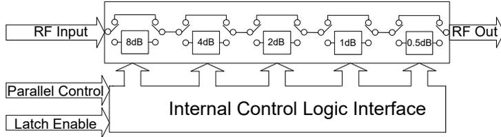
The ZX76-15R5A-PNS+ parallel interface consists of 5 control bits that select the desired attenuation state, as shown in Table 1: Truth Table.
