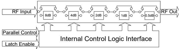
The ZX76-15R5A-PPS+ serial interface consists of 5 control bits that select the desired attenuation state, as shown in Table 1: Truth Table.
