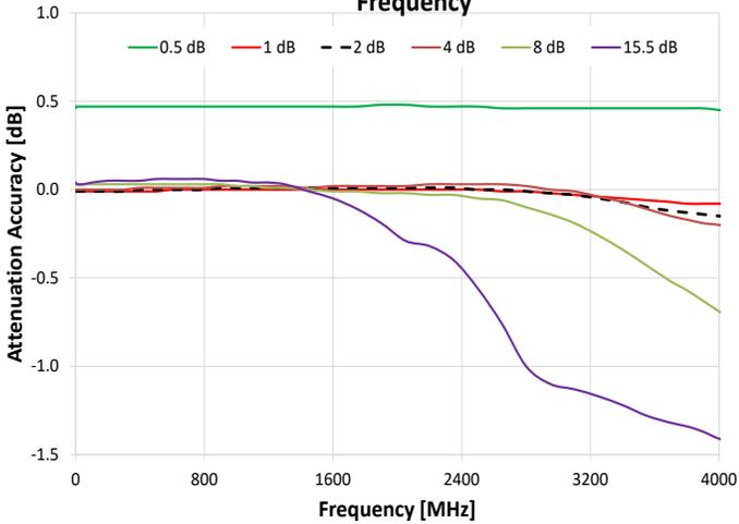
Attenuation relative to Insertion Loss vs. Frequency
