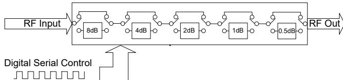
The ZX76-15R5A-SNS+ serial interface consists of 5 control bits that select the desired attenuation state, as shown in Table 1: Truth Table.
