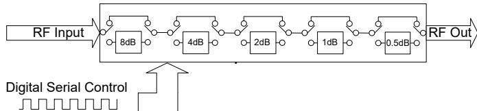
The ZX76-15R5A-SPS+ serial interface consists of 5 control bits that select the desired attenuation state, as shown in Table 1: Truth Table.
