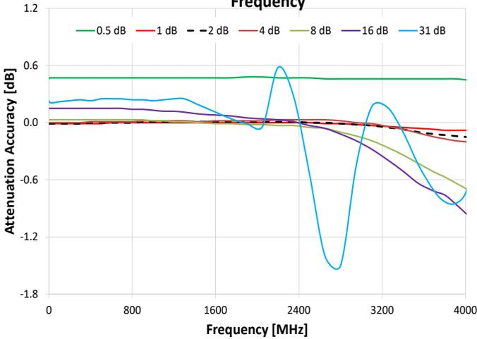
Attenuation relative to Insertion Loss vs. Frequency
