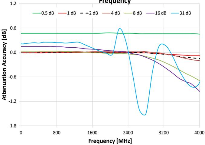
Attenuation relative to Insertion Loss vs. Frequency
