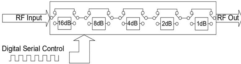
The ZX76-31A-SNS+ serial interface consists of 5 control bits that select the desired attenuation state, as shown in Table 1: Truth Table.
