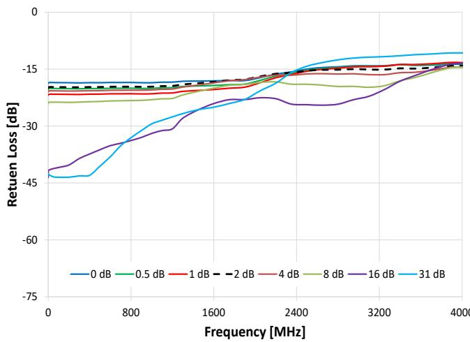
R. Loss Out vs. Frequency over Attenuation settings
