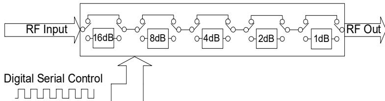
The ZX76-31A-SPS+ serial interface consists of 5 control bits that select the desired attenuation state, as shown in Table 1: Truth Table.
