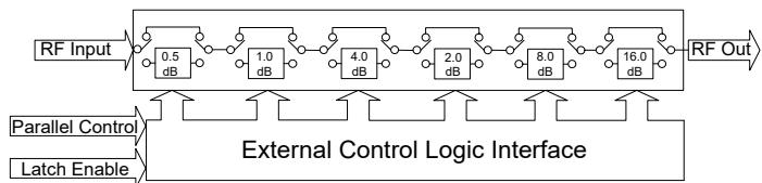
The ZX76-44G-30-K+ parallel interface consists of 6 control bits that select the desired attenuation state, as shown in Table 1: Truth Table.
