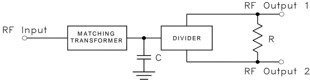
Figure 1 shows a block diagram of a power splitter. It consists of an input matching section, a divider section, a capacitor and a resistor. In a 50-ohm system, the impedance at the input of the divider is close to 25 ohms. The matching transformer converts this to 50 ohms at the RF input to provide a good match. Normally a capacitor C is required to match the reactive part of the impedance. The resistor R plays a critical role in providing isolation between the two RF out ports.
