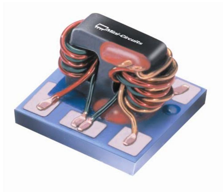
Fig 2. Photograph of the Miniature Power Splitter
