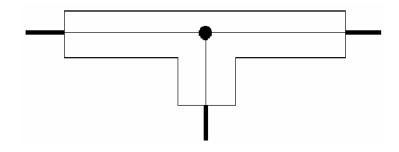
Fig. 2. Basic 2 way 0° power splitter, simple "T".
