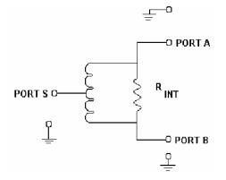
*Fig. 3. In a two-way splitter/combiner,* equal and opposite currents flow through the internal resistor and transformer, cancel each other, and provide high isolation between ports A and B.
