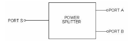
Fig. 1. When used as a  $0^{\circ}$  power splitter, the input is applied to port S and equal outputs appear at ports A and B. When used as a power combiner, both inputs are applied to ports A and B and the sum taken from port S.
