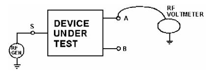
*Fig. 5. To improve insertion loss measurement*, first a 3dB standard attenuation is placed between points A and S, and an RF voltmeter reading is taken. Then the attenuator is removed and the power splitter/combiner is connected to A, B, and S.
