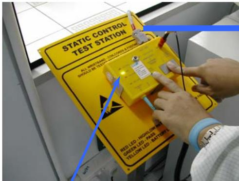
A green test indicator light means the wrist-strap is worn properly and is working as intended. This picture shows the configuration for testing wrist-straps. The test station can also be configured to test antistatic footwear.
