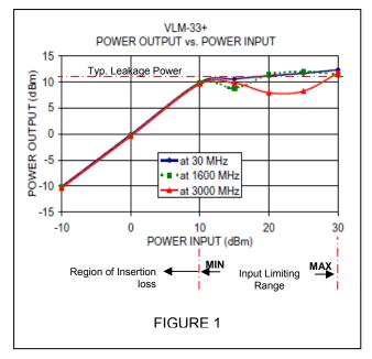
$\Delta$ output  $\Delta$ input characterization. For input signals above the maximum input power, the output will begin to increase again at a greater slope.
