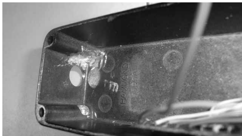
Figure 7 — I used a Hammond 1590A cast aluminum enclosure and had to remove some material from the corners to make room for the Mini-Circuits sensor. I center punched the area and then used my drill, being careful not to engage it and go through the wall. The probe SMA hole offset is to provide clearance for the LCD in the other side of the box. Not shown here, there was a hole drilled on the box “floor” to secure one of the sensor legs.
