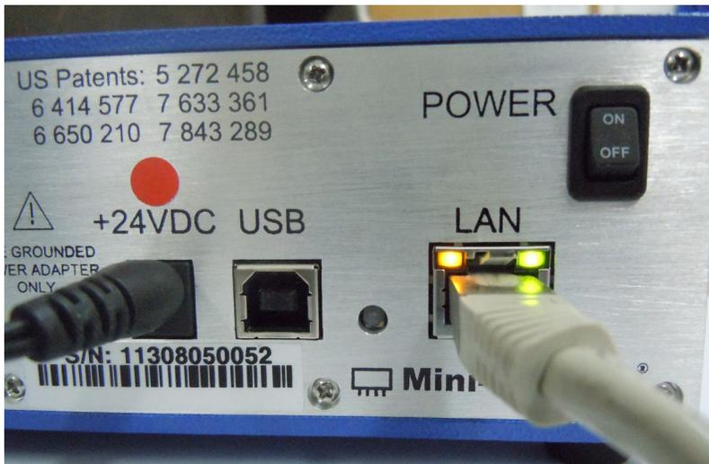
**Figure 2.3.3b:** switch matrix power & Ethernet control connections
