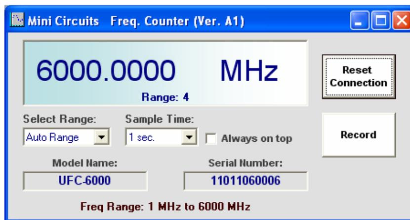
**Figure 3.2.4:** Frequency Counter Software Main Screen
