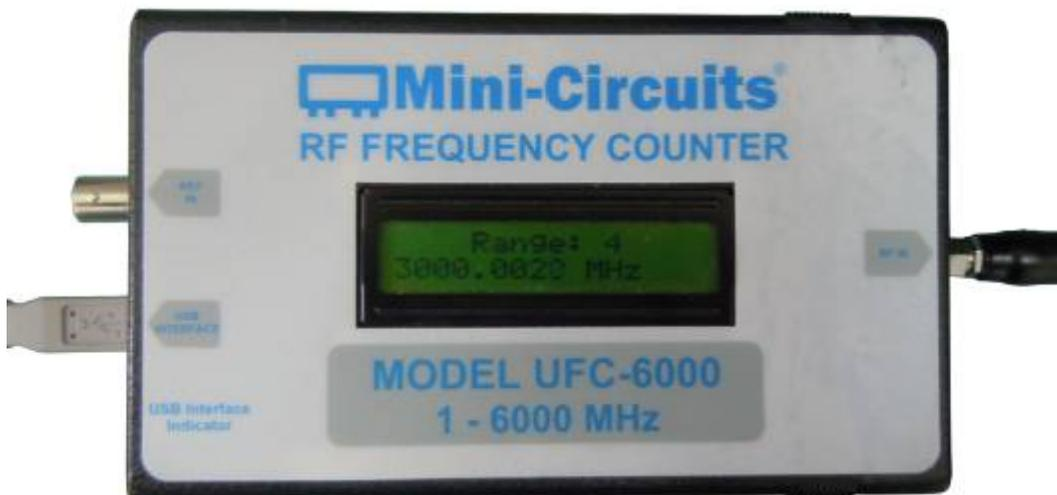
**Figure 3.1.4** UFC-6000 with internal reference testing D.U.T
