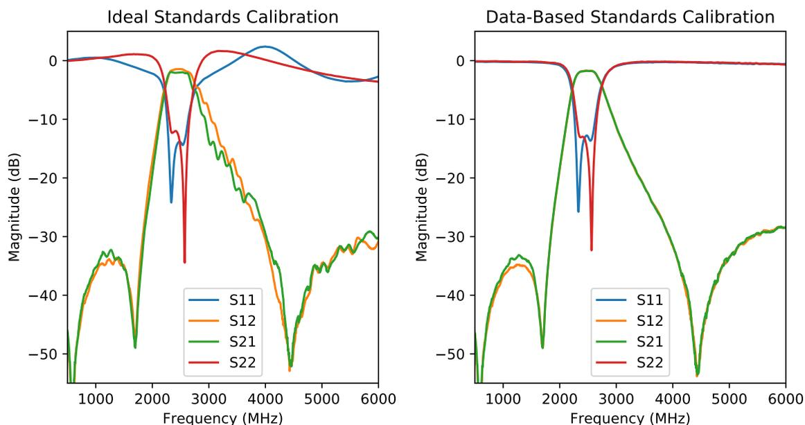
Figure 1: UVNA-63 kit measurement of a 2.5 GHz bandpass filter with ideal SOLT calibration (left) and data-based SOLT calibration (right)
