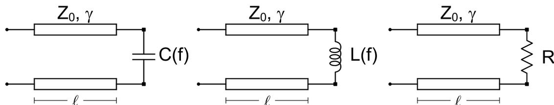
Figure 2: Transmission line model for open, short, and load terminations
