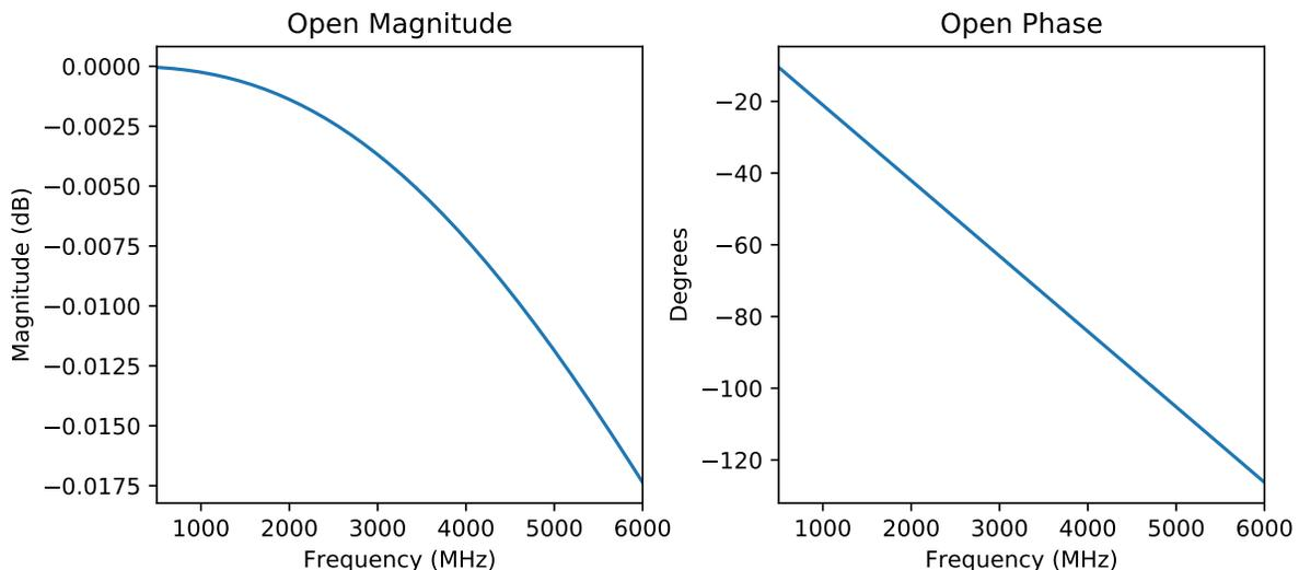
Figure 3: Model for the 85033D/E Cal. Kit Open Standard, Magnitude (left), Phase (right)
