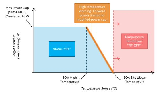
The above figure provides a visualization of the max power cap derating defined by the Temperature SOA. Power throttling provides a graceful degradation of performance that will allow continuous operation without damage or interruption.
