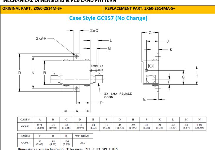
Dimensions are in inches (mm). Tolerances: 2Pl.  $\pm$ .03; 3Pl.  $\pm$ .015 Tolerance on hole size and interaxes dimensions to be  $\pm$ .005.
