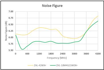
Please note that data compiled above is for ZHL-42WX+ and ZHL-10M4G21W0X+ (models without heatsink). Similar performance can be expected between the model supplied without heatsink and the model supplied with heatsink.
