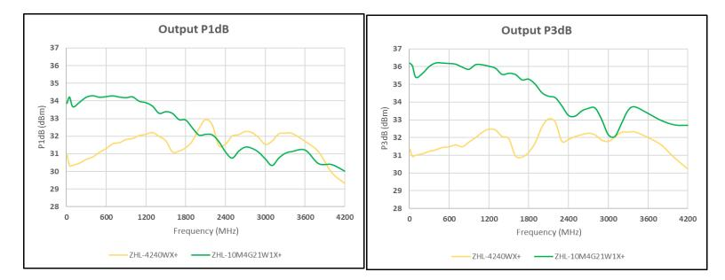
Please note that data compiled above is for ZHL-42WX+ and ZHL-10M4G21W0X+ (models without heatsink). Similar performance can be expected between the model supplied without heatsink and the model supplied with heatsink.
