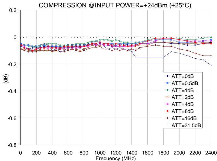
Fig. 5: Compression at +24 dBm input power
