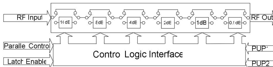
Fig. 9: Functional schematic of a 6 bit attenuator with parallel control.
