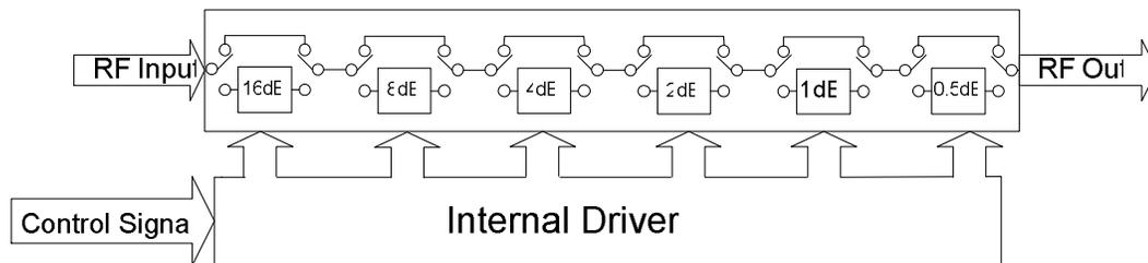
Fig. 1: Simplified schematic of a 6 bit digital attenuator.
