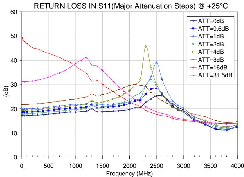
Fig. 4: Input return loss vs. Frequency
