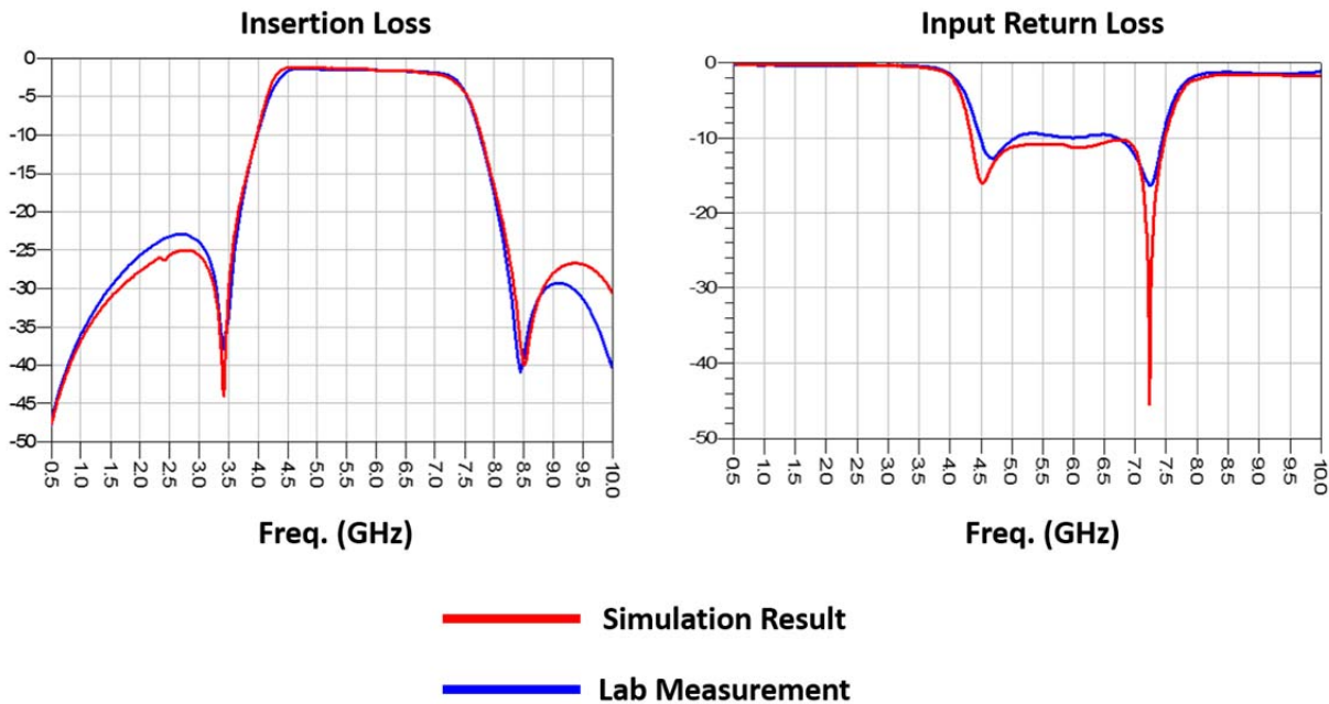
Figure 5: Advanced simulation of S21 and S11 of an LTCC bandpass filter model versus measured performance after first spin.
