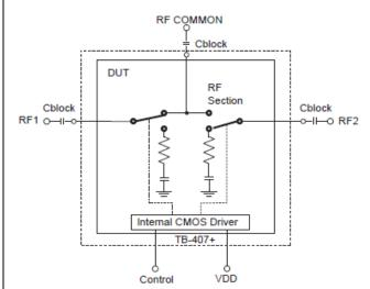
All RF connections must be DC blocked or held at 0V DC.
