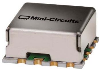
Figure 5: Model ROS-4608CH-2+ is a surface-mount VCO with fixed-frequency output at 4608 MHz with typical tuning sensitivity of 6 MHz/V for a control voltage range of 0.9 to 4.35V.
