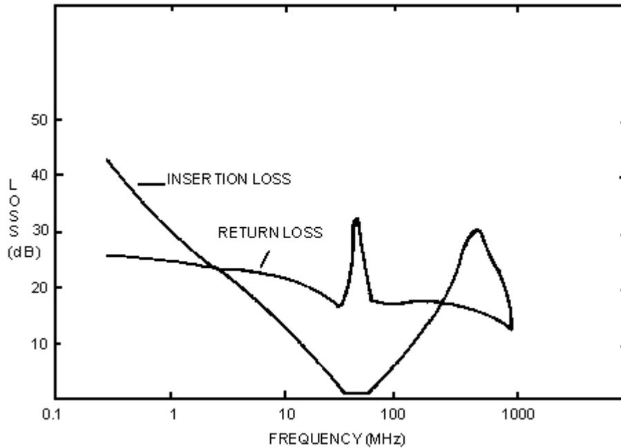
5. Insertion loss and return loss of a model PIF-40 IF filter are plotted.
