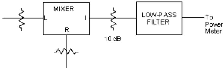
1. The mixer conversion loss measurement setup is diagramed.
