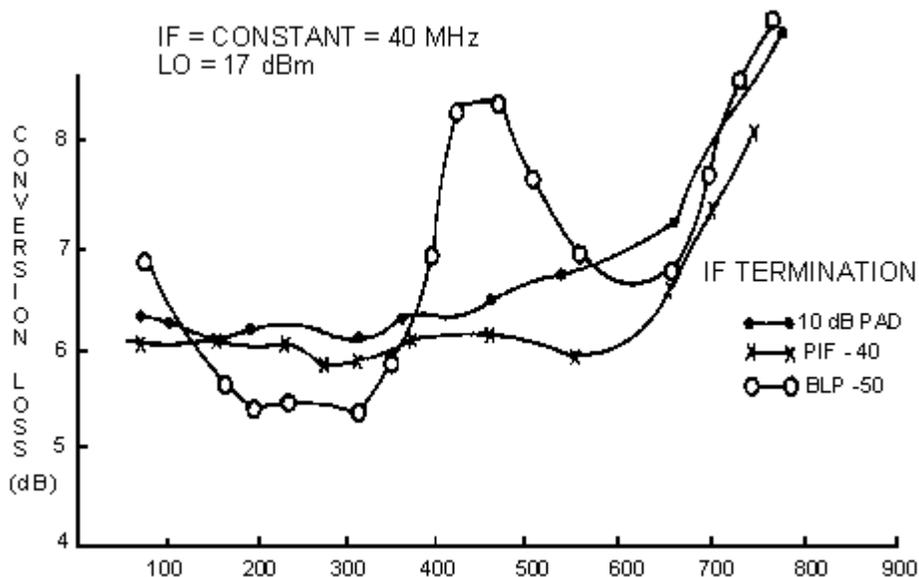
4. Conversion loss is shown as a function of the IF filter.
