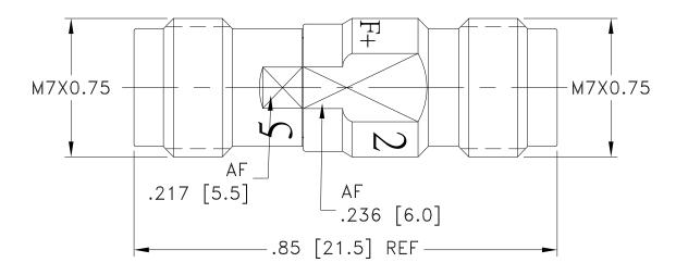
Weight: 3.8 grams Dimensions are in inches (mm). Tolerances:  $2 \text{ Pl.} \pm .030$ ; 3 Pl. + .015
