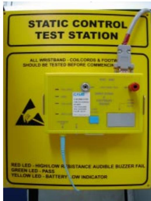
A green test indicator light means the wrist-strap is worn properly and is working as intended. This picture shows the configuration for testing wrist-straps. The test station can also be configured to test antistatic footwear.
