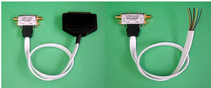
Connectorized DAT attenuator ZX76-31R5-PN attenuator with parallel control cable and connector (left) and without interface connector (right)
