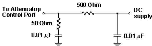
At RF frequencies greater than 1 MHz, the capacitors act like a short and the 50 and 500 ohm resistors appear in parallel, which is almost 50 ohm. For dc and low frequencies, the capacitor is nearly an open. Hence, dc current is applied through 500 ohms from the dc power supply.
