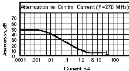
Attenuation vs frequency is a function of the control current; the higher the control current level, the flatter the response.
