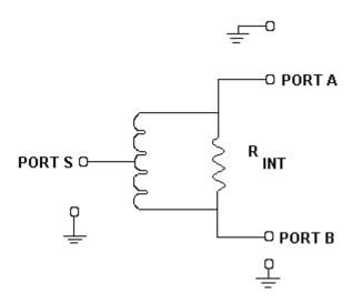
2. *In two-way splitter/combiner*, equal and opposite currents flow through the internal resistor and transformer, cancel each other, and provide high isolation between ports A and B.
