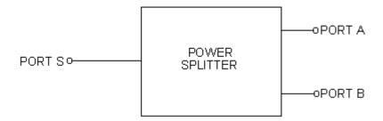
1. When used as a  $0^{\circ}$  power splitter, the input is applied to port S and equal outputs appear at ports A and B. When used as a power combiner, both inputs are applied to ports A and B and the sum taken from port S.
