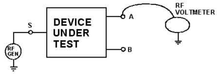
**3.** To improve insertion loss measurement, first a 3dB standard attenuation is placed between points A and S, and an RF voltmeter reading is taken. Then the attenuator is removed and the power splitter/combiner is connected to A, B, and S.
