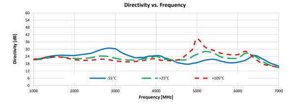
Test Conditions: Input Power = +5 dbm, Configuration B.
