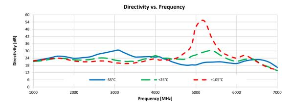
Test Conditions: Input Power = +5 dbm, Configuration A.
