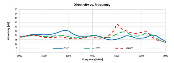
Test Conditions: Input Power = +5 dbm, Configuration D.
