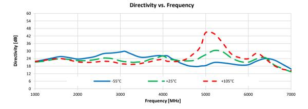
Test Conditions: Input Power = +5 dbm, Configuration C.
