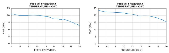
Note: All data taken in this section represents the Die attached in a 4x4 mm 24-Lead QFN-style package and measured on Mini-Circuits Characterization Test Board TB-LVA-6183PNC+. All data taken at nominal conditions V<sub>CC</sub> = +6 V, V<sub>C</sub> = +6 V, and V<sub>B</sub> = +5.4 V unless noted otherwise. For over voltage data, see LVA-6183PN+.
