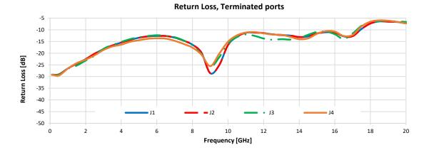
Test Conditions: @ Temperature = +25°C, Pin = 5 dBm.
