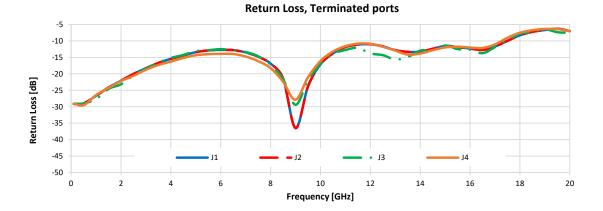
Test Conditions: @ Temperature = +60°C, Pin = 5 dBm.
