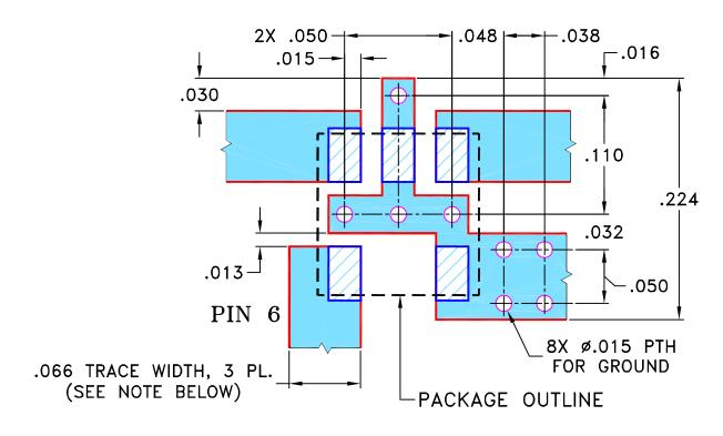
NOTES: 1. TRACE WIDTH IS SHOWN FOR ROGERS RO4350B WITH DIELECTRIC THICKNESS .030"  $\pm$  .002"; COPPER: 1/2 OZ. EACH SIDE. FOR OTHER MATERIALS TRACE WIDTH MAY NEED TO BE MODIFIED.
