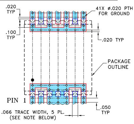
NOTES: 1. TRACE WIDTH IS SHOWN FOR ROGERS RO4350B WITH DIELECTRIC THICKNESS .030"  $\pm$  .002"; COPPER: 1/2 OZ. EACH SIDE. FOR OTHER MATERIALS TRACE WIDTH MAY NEED TO BE MODIFIED.
