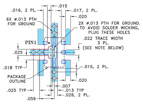
NOTES: 1. TRACE WIDTH IS SHOWN FOR ROGERS RO4350B WITH DIELECTRIC THICKNESS .010"  $\pm$  .001"; COPPER: 1/2 OZ. EACH SIDE. FOR OTHER MATERIALS TRACE WIDTH MAY NEED TO BE MODIFIED.
