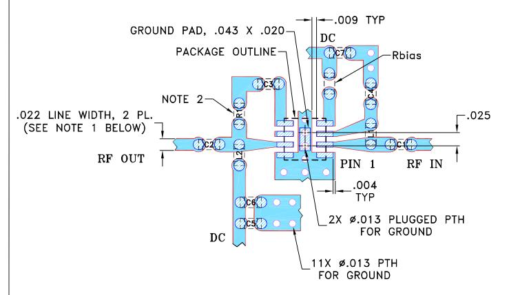
NOTES: 1. TRACE WIDTH IS SHOWN FOR ROGERS RO4350B WITH DIELECTRIC THICKNESS .010"  $\pm$  .001"; COPPER: 1/2 OZ. EACH SIDE. FOR OTHER MATERIALS TRACE WIDTH MAY NEED TO BE MODIFIED.
