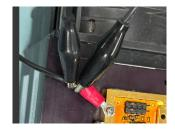
All Drains are tied together thru L1, L4, L2,L3 and a jumper cable connecting top and bottom Drains.
