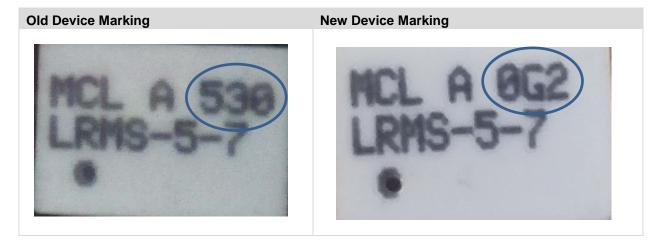
Note: This is an example of internal device marking for space limited products. This is for demonstration purposes only.
