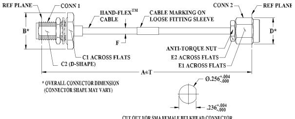
CUT OUT FOR SMA FEMALE BULKHEAD CONNECTOR PANEL THICKNESS .100 INCHES
