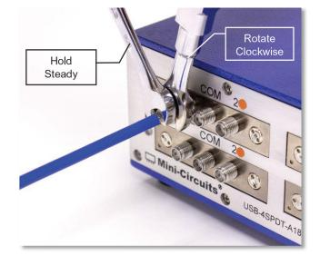
\*NOTE: Mini-Circuits recommends using a 5/16-inch open end wrench calibrated to 8 inch-pounds maximum torgue to prevent damage due to over-torqueing the connector.
