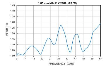
50Ω DC to 67 GHz Right-Angle 1.85 mm-Female to 1.85 mm-Male
