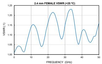
50Ω DC to 50 GHz Right-Angle 1.85 mm-Female to 2.4 mm-Female
