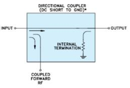
\* ELECTRICAL SCHEMATIC IS FOR DIRECTIONAL COUPLER WITH INTERNAL TRANSFORMER(S) THAT ROUTES DC FROM RF PORTS TO GROUND.
