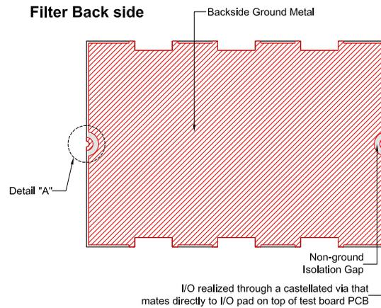
Filter RF I/O Detail (Filter Back Side)
