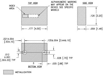
Weight: .126 grams. Dimensions are in inches [mm]. Tolerances: 2PI.±.01; 3PI.±.005
