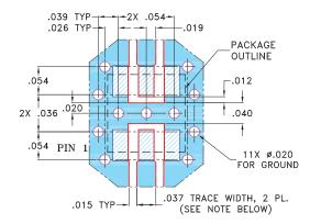
NOTES: 1.TRACE WIDTH IS SHOWN FOR ROGERS RO4350B WITH DIELECTRIC THICKNESS 0.020"  $\pm$  0.0015"; COPPER: 1/2 OZ. EACH SIDE. FOR OTHER MATERIALS TRACE WIDTH MAY NEED TO BE MODIFIED.
