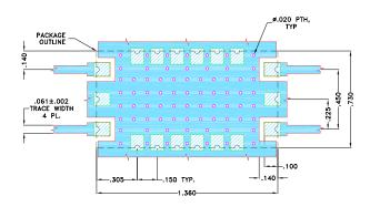
NOTES: 1. TRACE WIDTH IS SHOWN FOR OAK-602, WITH DIELECTRIC THICKNESS .022"±.0015". COPPER: 1/2 Oz. EACH SIDE. FOR OTHER MATERIALS TRACE WIDTH MAY NEED TO BE MODIFIED. 2. BOTTOM SIDE OF THE PCB IS CONTINUOUS GROUND PLANE. DENOTES PCB COPPER LAYOUT WITH SMOBC (CONTENT WICK OWER BASE CORPER) (SOLDER MASK OVER BARE COPPER)
